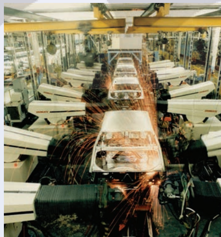
B Automation. Robots weld car bodies on a General Motors assembly line in Oshawa, Ontario, in Canada. Automation has been occurring for decades in North America and may account for more job losses in manufacturing than globalization. This photo was taken in 1985. [Keith Beaty/Toronto Star via Getty Images]
